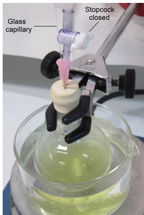
Fig 4.2.4.2.7 Taking a sample for TLC with a glass capillary
