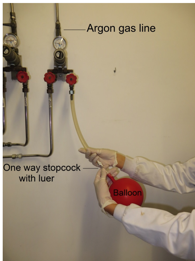
Fig 4.2.4.2.3 Filling the balloon with argon gas
