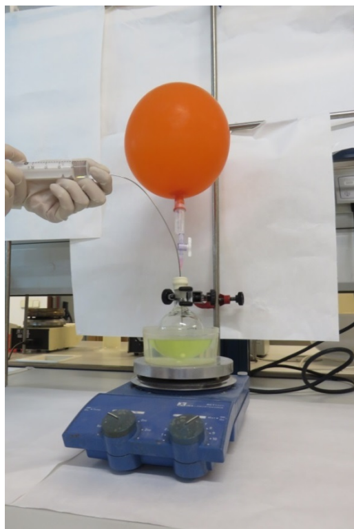
Fig 4.2.4.2.5 Transfer MeLi to the reaction flask
